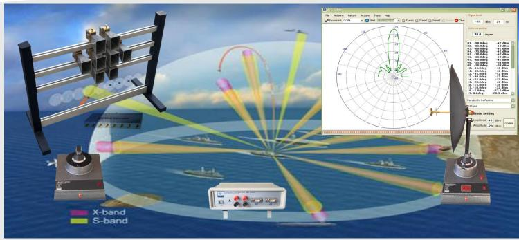
PAT-5000 is completely computerized antenna array training system that performs PC based automated rotation of receiving antennas at predefined angles and GUI-based polar plots of radiation patterns of each antenna. PAT-5000 comprises of C-Band microwave transmitter receiver and set of eight element Horn antennas. It is a low cost high performance antenna arrays training system that is also used as a design tool for those engaged in research and development of projects in the field of antennas.
