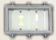
Most of the components are packaged in bright aluminum enclosures and their interconnection is by standard SMA couplings; providing secure but easily made joints.
